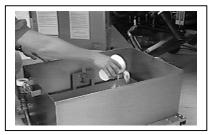
8. Sprinkle 16oz of filter powder onto filter paper in filter pan. Make sure top filter sheet is covered evenly.
