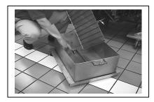
5. Lift out protection screen and clean around the nipple in the pan bottom.
