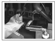
4. Pull the yellow oil return handle out to open return line to the fryer. Turn filter switch "ON" to begin pumping clean oil back into the fryer. Allow the oil to flow for a few seconds to wash out sediment in the bottom of the cooking vessel.
