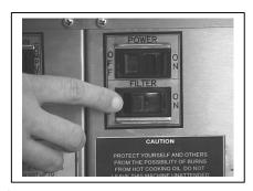
6. Allow the pump to run for 20 -30 seconds after air bubbles appear in the fryer vessel before shutting off to clear shortening/oil from the return lines. Turn filter switch "OFF" after all the oil has been pumped back into the fryer. Push the yellow oil return handle in.
