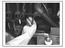
3. Remove screen from fry vessel. Mix crumbs and oil by stirring with a brush. Open the drain valve by pulling the red handle out. Then oil will drain from the fry vessel into the filter pan.
