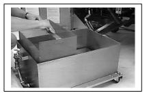
4. Remove filter pan cover and crumb tray. Visually inspect filter paper sheets. Scrape debris off top filter sheet. Remove hold-down ring. Discard top sheet if scuffed or darkened.
