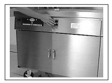
1. Turn fryer OFF. If fryer has an oil return line heater and solid shortening is used, turn the filter switch to the heater position for a few minutes to melt solid shortening in the pump lines before filtering.
